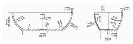
BAT-CHA-MRF-FSD-DWH-0TH Size: L1680mm x w800mm x h500mm
