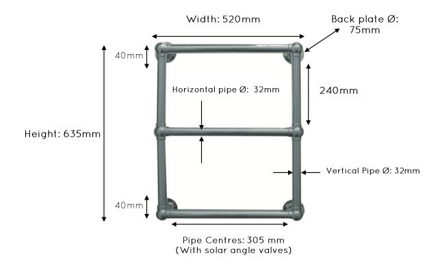
Overall Projection: 150mm Pipe Centres from the Wall: 50mm
