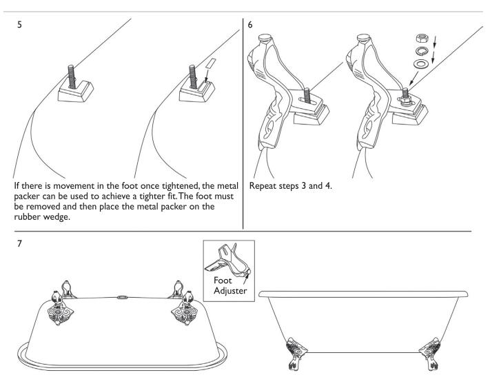
Once all feet are securely attached, the bath can be turned over. The bath is heavy, so adequate manpower is required to avoid injury. If the bath is on uneven ground, the foot adjusters can be turned to stabilise the bath.
