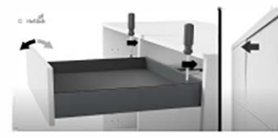
15° REGULATE THE DOOR'S INCLINATION
