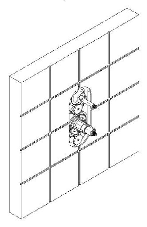
1. Install the finished surface, ensuring the finished surface is in accordance with the minimum and maximum installation depths shown on the drawings in the front of this booklet.
