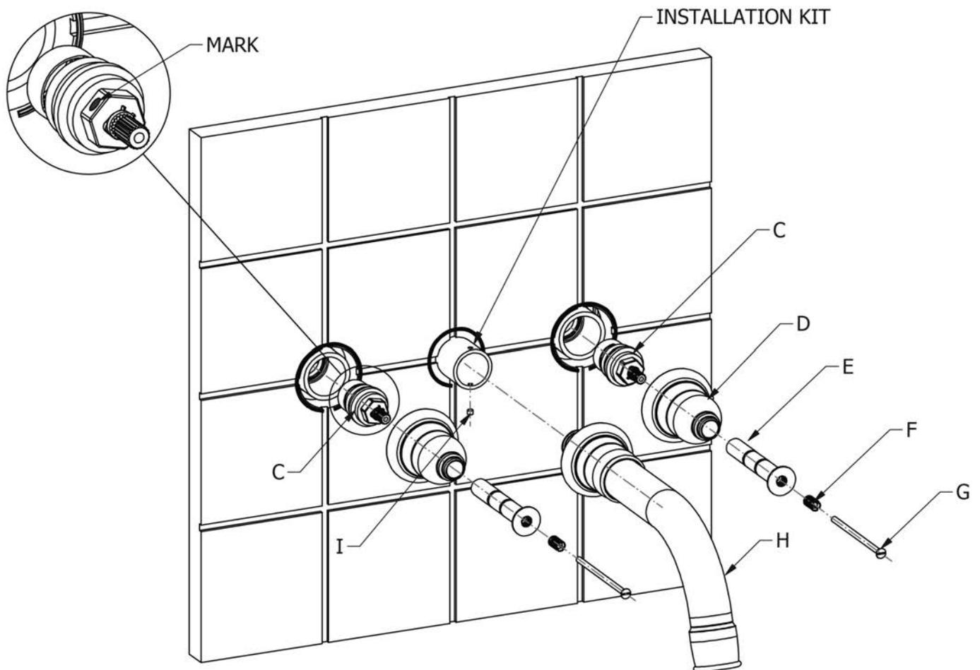
4. Screw in CD valves (C) into the installation kit ensuring that the left CD valve has the mark as shown. Ensure valves are fully tightened.
