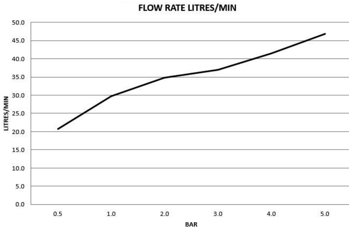
The flow rate data provided in this document is indicative of each product and is given in an open outlet condition. Installation design, external connections and fittings not supplied may affect the data provided.
