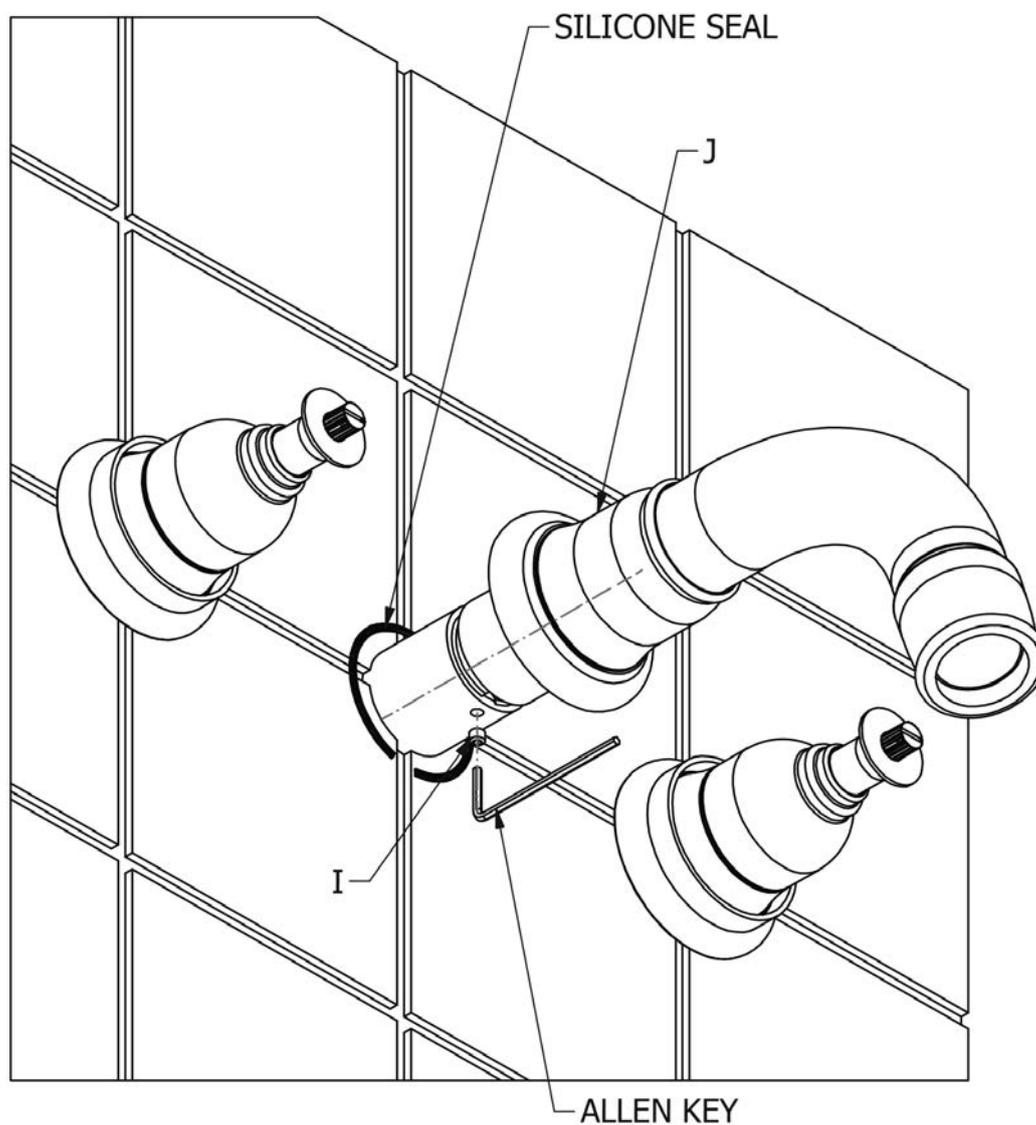
8. Apply a suitable silicon sealant to the wall where the spout body (J) will sit. Slide spout body (J) over spout assembly (H) and secure using grub screw (I) with Allen Key. Ensure grub screw is fully tightened.
