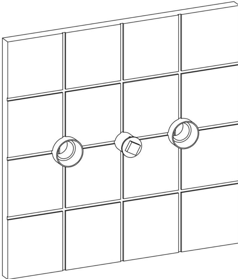
1. Install the finished surface, ensuring the finished surface is in accordance with the minimum and maximum installation depths shown on the drawings in the front of this booklet.
