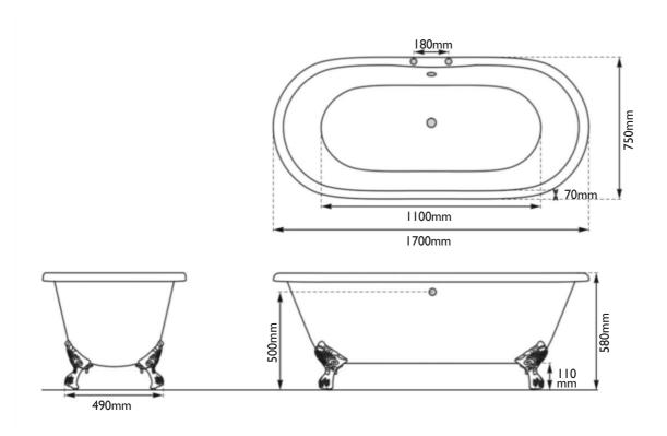
The Washington: a double ended cast iron bath with a vitreous enamel interior, exterior painted in Mid-French Grey as standard, ready to install. This bath comes complete with ball and claw cast iron feet painted in Soft White available with 2 tap holes.
