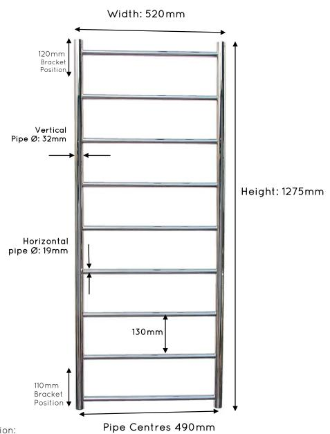
Overall Projection: 117mm\* Pipe Centres from the Wall: 102mm \*When using short brackets, projection and pipe centres from wall will be reduced by 25mm.
